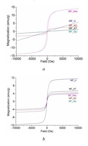
Fig. 3 – Magnetization as a function of applied field loops of FeMnO<sub>3</sub> powders sintered at: a) 500°C and b) 1200°C.
