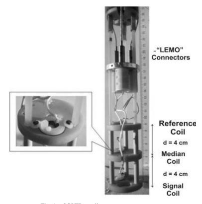
Fig. 1 – SQUID gradiometer.
