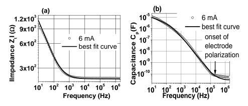
Fig. 6 – Typical fitting curves to determine the unknown parameters  $C_{dl0}(j)$ , n,  $R_{F0}(j)$  and m.
