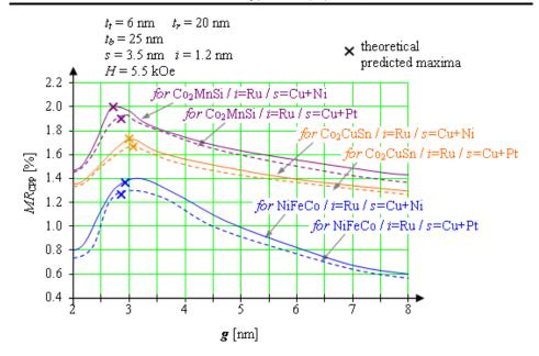
Fig. 2 – The CPP magnetoresistance ratio of the considered spin valves in function of the average grain size of the hard magnetic layer. Simulational and theoretical maxima were illustrated on graphs.
