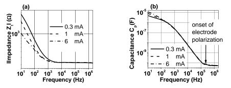
Fig. 4 – *a*) The impedance modulus  $IZ_t(f,j)I$  measured with the DBS electrode in physiologic saline for three values of the current: 0.3, 1 and 6 mA (current density 5 to 100 mA cm<sup>-2</sup>); *b*) The equivalent parallel capacitance  $C_p(f,j)$  of the DBS electrode measured in the same conditions as above.
