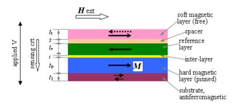
Fig. 1 – The considered layers configuration in the spin valve head. Sensing current flows perpendicular to the ferro / nonferro-magnetic interfaces, in the current-perpendicular-to-plane (CPP) geometry.
