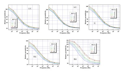
Fig. 4 – Frequency dependence of the relative permittivity at room temperature in the relative humidity range 0–100%.
