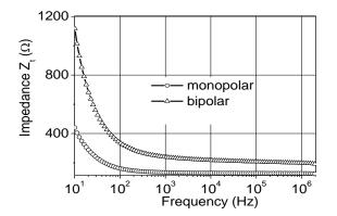
Fig. 5 – The absolute value of the impedance of the DBS electrode in 0.9% NaCl saline for the case of monopolar (circles) and bipolar (triangles) configuration. The applied voltage was 1V rms.
