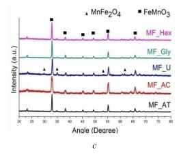
Fig. 2 – XRD patterns (color online) of iron manganese oxides powders synthesized with different agents and annealed at different temperatures: *a*) 500°C, *b*) 900°C and *c*) 1200°C.
