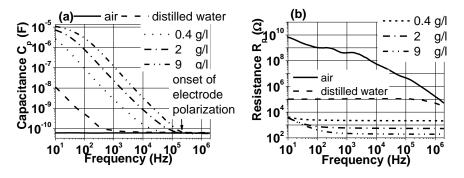
Fig. 3 – *a*) The equivalent parallel capacitance  $C_p(f)$  of the DBS electrode. The arrow indicates the onset of electrode polarization. The onset frequency is lower as the saline concentration is lower; *b*) The equivalent parallel resistance  $R_p(f)$  of the DBS electrode. Above a certain frequency which increases with saline concentration  $R_p$  is
