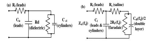
Fig. 2 - a) The equivalent circuits of the DBS electrode in air for the case of bipolar configuration; *b*) The equivalent circuits of the DBS electrode in saline solution for the case of bipolar configuration.
