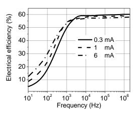
Fig. 7 – The electrical efficiency  $\eta(f)$  for three values of the current. The electrical efficiency is frequency dependent.
